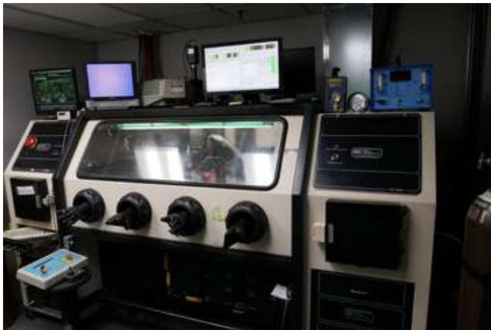
Glove box controlled environment typically used for laser hermetic sealing applications.
